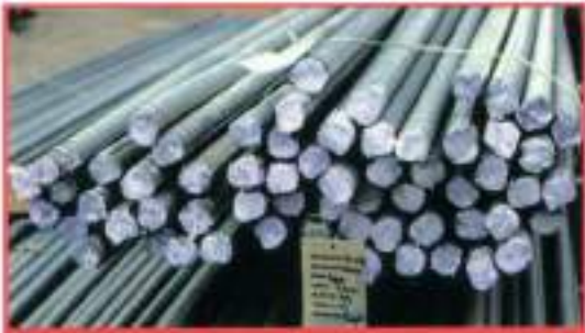
7 Metres cut to length bars ready for delivery
